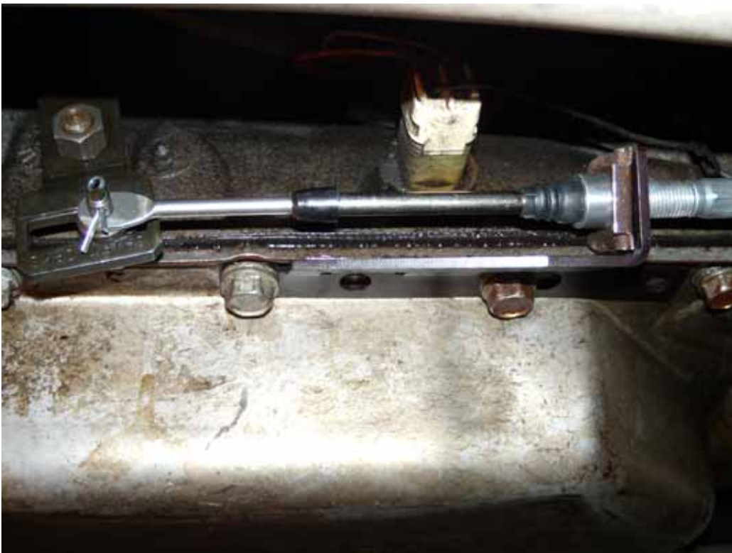
Cable installed at transmission
