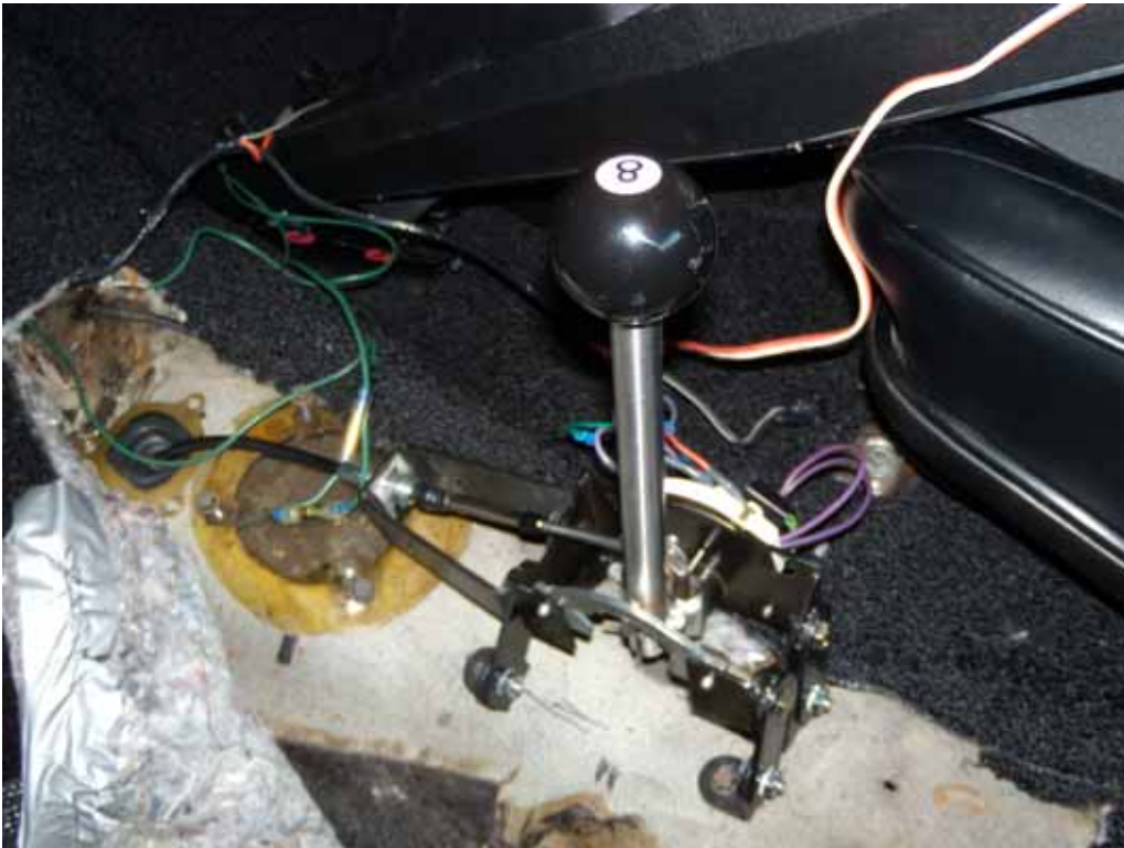
Shifter installed in car. Note original large hole in floor from Powerglide shifter, and location of cable exit hole in floor. Exit hole is about 5 ½ inches from forward point of shifter.
