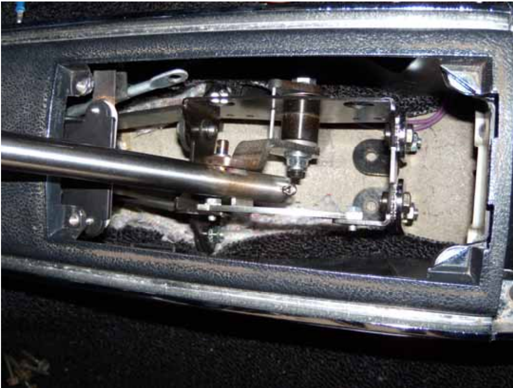
Locating shifter on tunnel with console as guide
